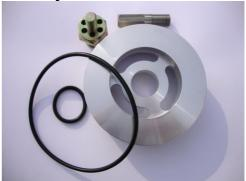
Remove the bowl which contains the original oil filter element and place to one side. Remove the old rubber seal which sits in the groove in the filter head. This may be difficult to see and it often seems as though there is no seal as they become hard and compressed with age, but it is important to replace this seal in order to ensure a leak-proof installation.
